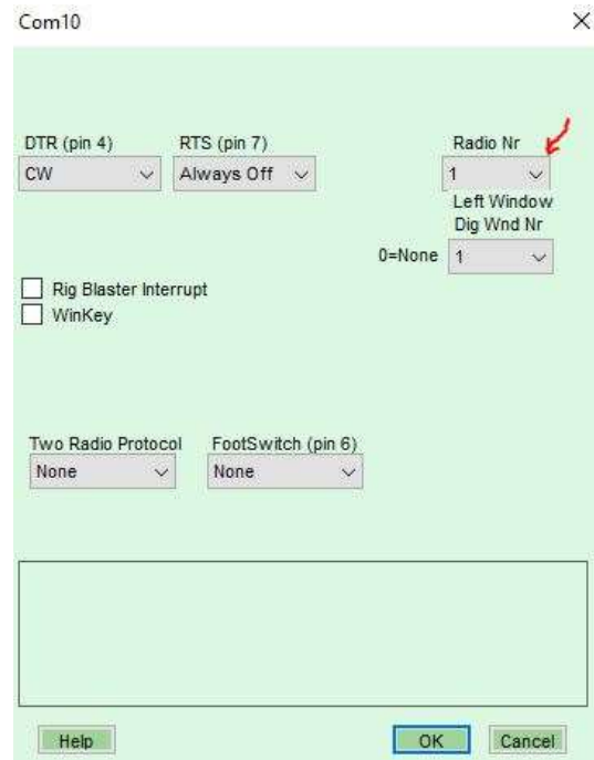
Setting up the FTDX-10 on the Standard port for CW. Select DTR = CW Select Radio Nr 1.
